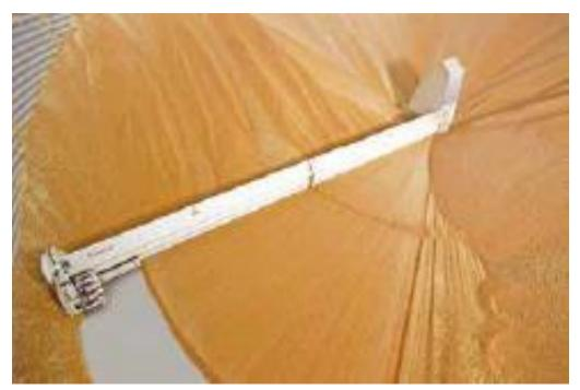
It is used to completely empty the flat bottom silo.
